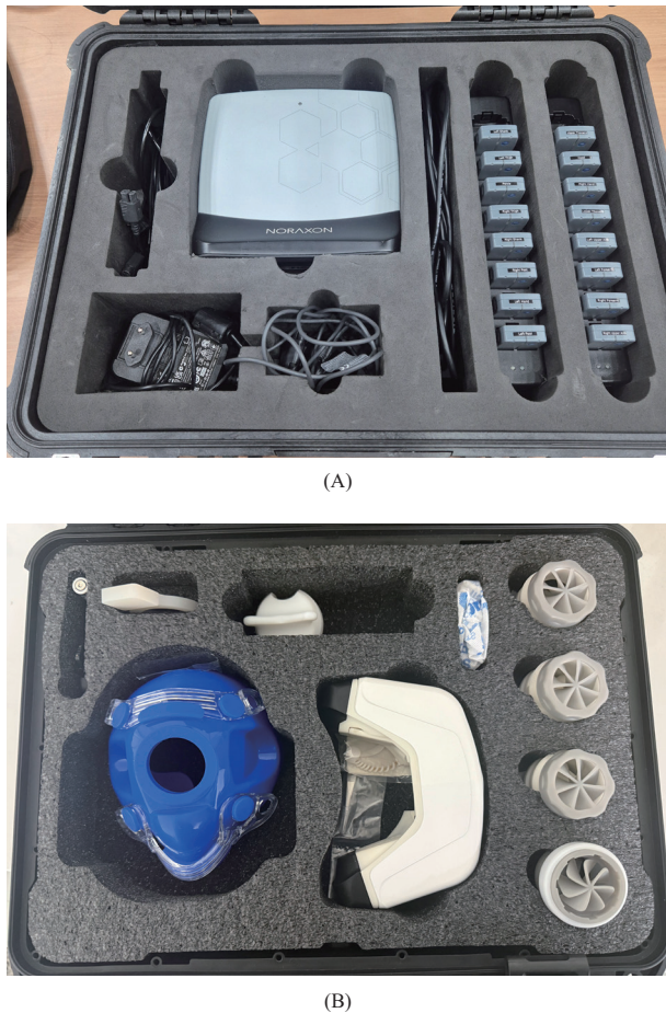
Fig. 2. Experimental equipment. (A) Inertial measurement unit (IMU) sensor (B) Portable VO 2 analyzer
