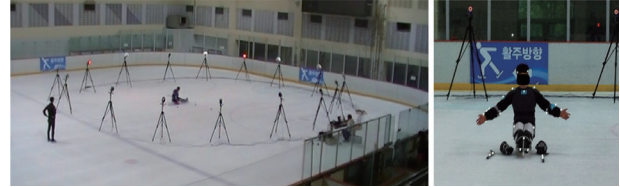
Fig. 2. Installation of an infrared camera (left) and marker attachment for motion analysis of a para-ice sledge hockey athlete (right)
