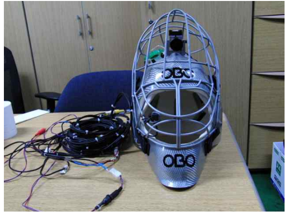
Fig. 1. eye tracking system for field hockey goalkeeper
