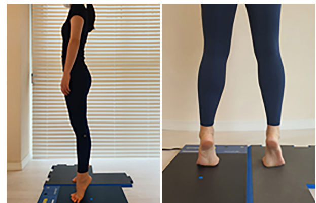
Fig. 1. Measurement of Foot Pressure Distribution during heel raise
