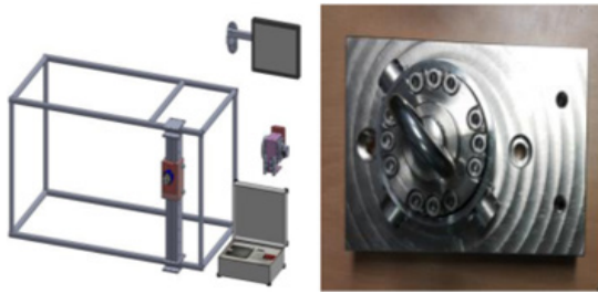
Fig. 2. Structure of force vector equipment (left) and load cell sensor (right)
